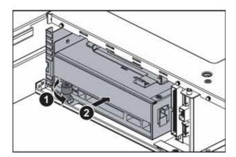
7 Lift the locking tab (3) on the back of the optical drive tray, then push the optical drive (4) and tray out of the bay.
